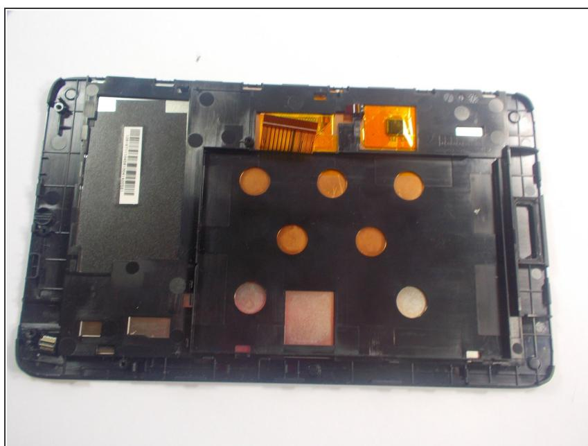
*i* With the logic board removed the old screen is all that remains. Reassemble using a new screen as the base.
